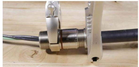
The hex-shaped portion of the connector's barrel is the ideal place to hold the barrel and prevent it from rotating while the nut is tightened. If needed, the inspection port plugs can be removed using a flat-head screw driver to allow a wrench to be used at this location without any interference.
