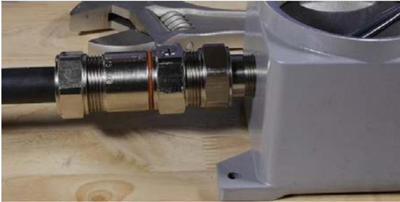
Again, insure that the connector's barrel is not rotated. All rotation should be made at the hub nut itself. This is done to ensure that the cable is not stressed.
