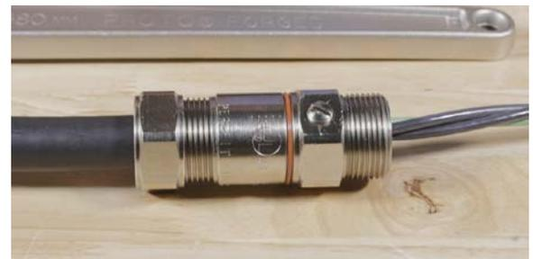
The connector should now be fully secured to the armor and the cable's outer jacket. If for some reason
