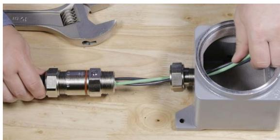
Hand-tighten the hub nut to the connector. Make sure that the nut is rotated during this process, and not the connector's barrel. Rotating the barrel may cause stress in the cable.
