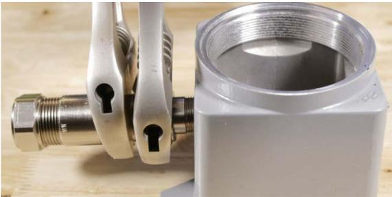
Once loose, the connector's barrel can be removed from the hub and the installation process can continue.
