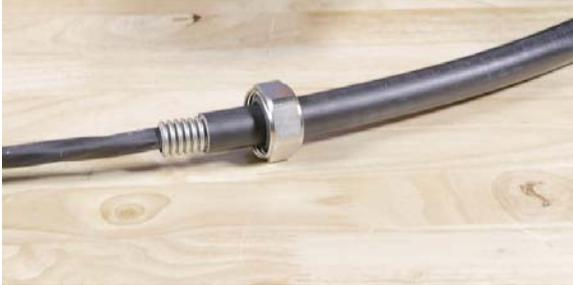
The nut and grommet should be slid about 2 inches [5 cm] past the end of the DekaFlex® armor so that they will not interfere with the connector's barrel. The seal may be snug, but should not require excessive effort to slide onto and along the outer jacket. Take care not to damage the outer jacket during this step.
