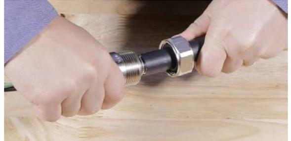
Now the connector can be tightened using a wrench. Make sure any rotation is limited to the grommet nut, and not the connector's barrel. Rotating the barrel could loosen the connector from the armor, resulting in a weak connection or faulty seal.
