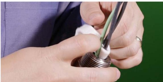
The damming fiber will prevent the sealant from flowing into the enclosure and will lessen the amount of sealant needed to fully seal the connector.
